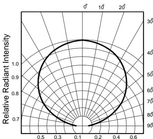
Fig.6 Radiation Diagram (Y-axis)
