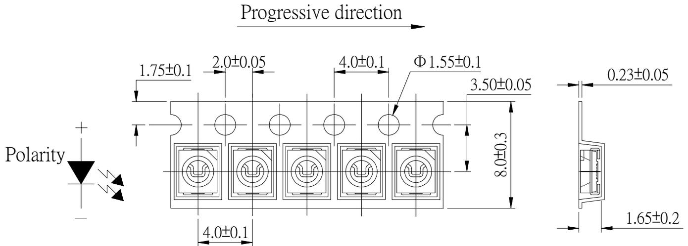
**Note:** Tolerance unless mentioned is  $\pm 0.1$ mm; Unit = mm
