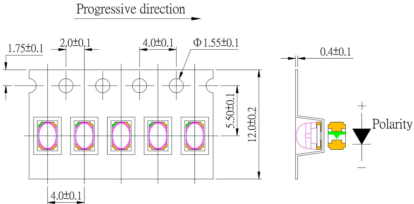
**Note:** Tolerance unless mentioned is  $\pm 0.1$ mm; Unit = mm
